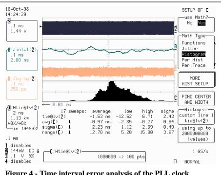
Figure 4 - Time interval error analysis of the PLL clock
