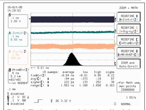
Figure 3 – Time interval error analysis of the working clock oscillator
