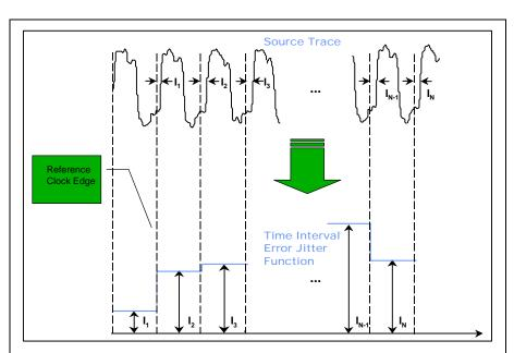
Figure 2- The Time Interval Error (TIE) JitterTrack function
