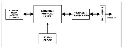
Figure 1 – Excessive clock jitter can cause missed data packets in Ethernet local area networks
